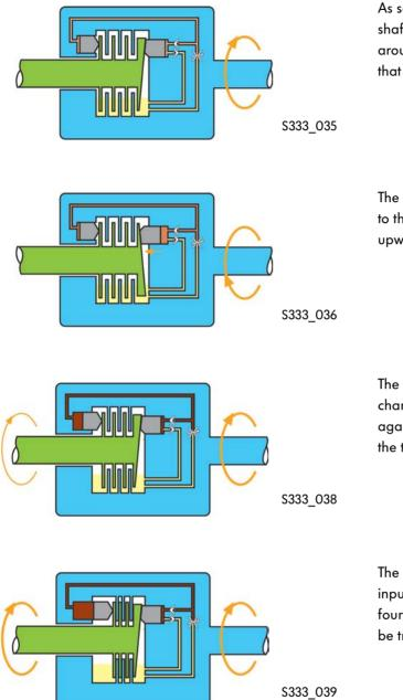
As soon as there are different wheel speeds, the input shaft turns with the actuating roller of the lifting piston around the lifting plate connected to the output shaft that is rotating at a lower speed.
