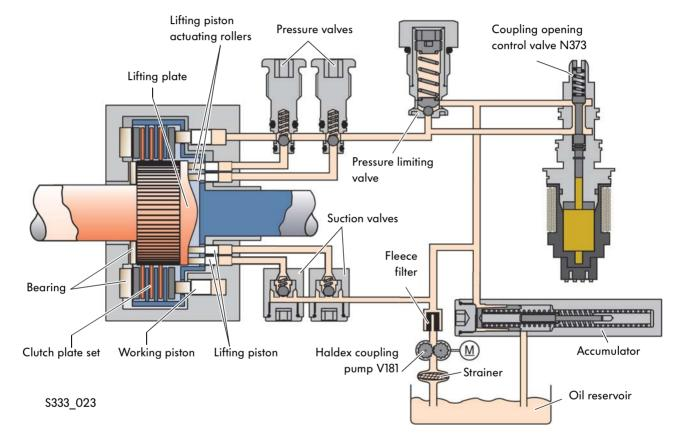
When the ignition is switched on and the engine does not issue a speed signal, the Haldex coupling system is pressure free. All valve springs are relieved. Pressure is built up again and another oil flow started.
