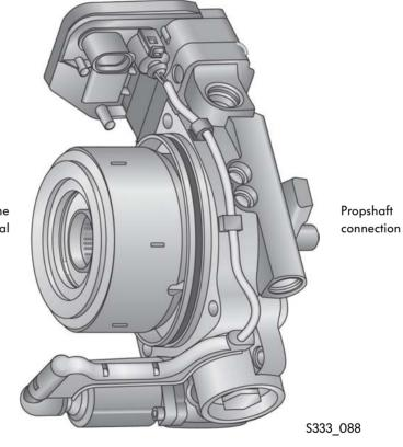
Hub for the shaft to the rear-axle differential
