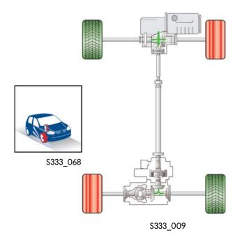
In theory, propulsion is not possible in this situation: There is no driving power at any of the wheels due to the power distribution of the axle differentials.
