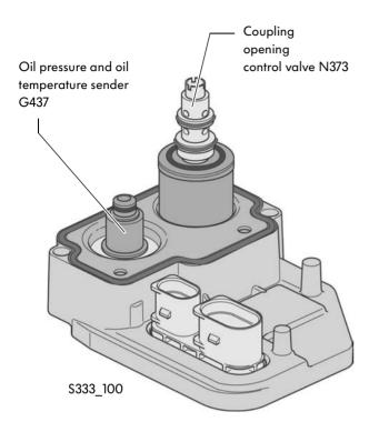
The four-wheel drive control unit J492 is always replaced together with the oil pressure and oil temperature sender G437 and the coupling opening control valve N373.
