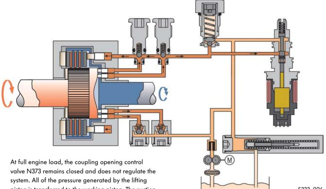
S333\_026 The maximum pressure in the system is defined by the pressure limiting valve: It opens at a pressure of 100 bar so that pressure is relieved through the channel via the accumulator into the oil reservoir.
