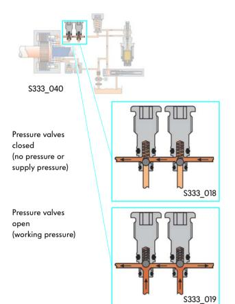
The pressure valves are located between the lifting piston, the working piston and the control circuit with the pressure limiting valve and the coupling opening control valve N373. They are spring-loaded and open when the supply pressure is exceeded.
