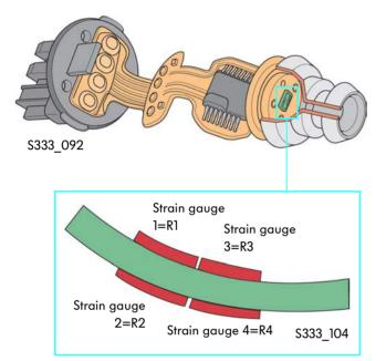
The oil pressure and oil temperature senders are in the same component.
