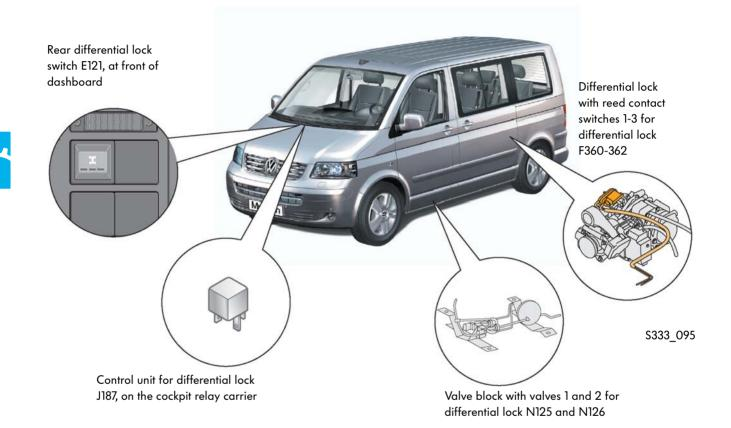
If the driver presses the differential lock button, the signal will be forwarded to the differential lock control unit J187. The differential lock control unit J187 receives the signal whether the conditions for switching on the differential lock are met from the differential lock control unit J104. If this is the case, it will operate differential lock valves 1 and 2 (N125 and N126) and the lock will be switched on.
