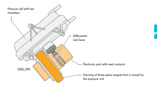
The voltage in the component changes according to the switch position and the four-wheel drive control unit J492 receives a signal about the state of the differential lock. Three different states are recognised.
