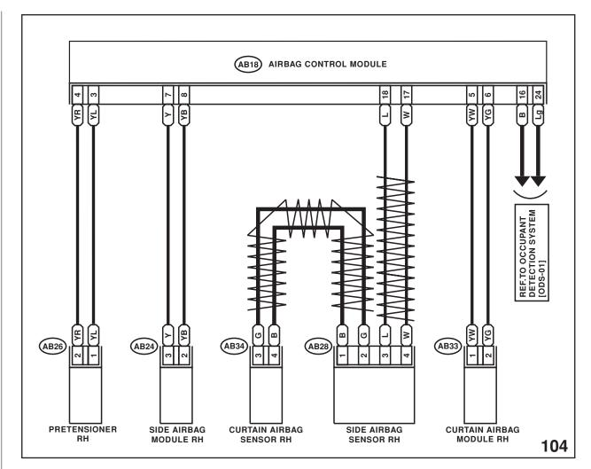
Airbag Wiring Schematic
