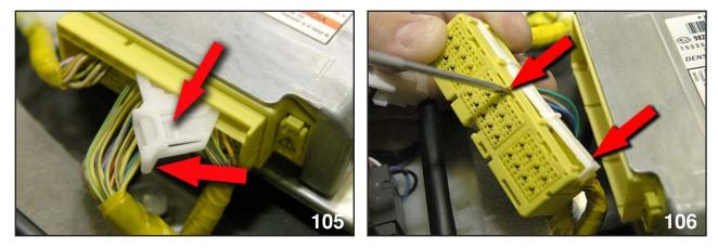
Connector Lock release tab
