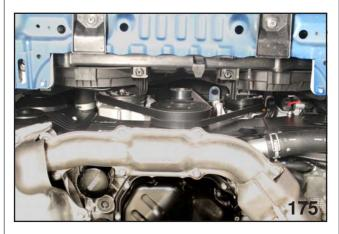
Air Conditioning Compressor Belt from under car
