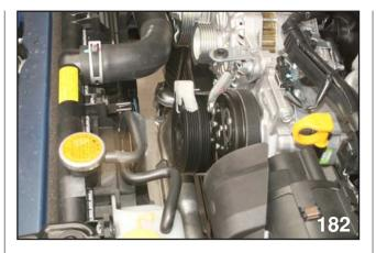
Belt Fully Engaged on Crankshaft Pulley Confirm belt is fully engaged on both pulleys.
