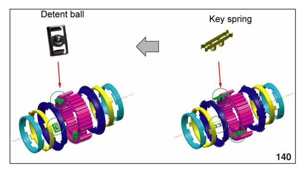
Difference of Detent Balls and Key Springs NOTE: Only two detent balls are used on the 1st and 2nd gear hub.
