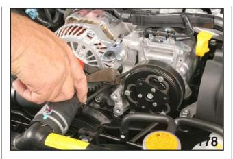
Cutting off Air Conditioning Compressor Belt
