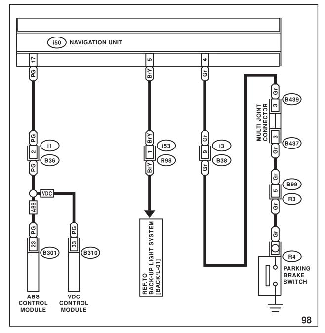
Navigation Unit Wiring Schematic
