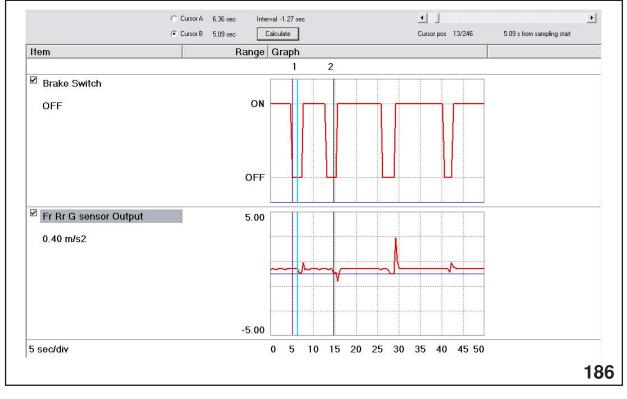
Brake Pedal Off and Brakes Releasing
