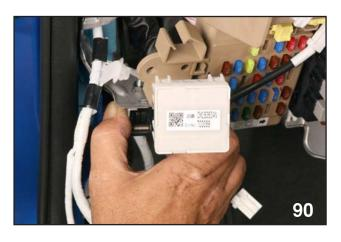
Releasing Multi Joint Connector
